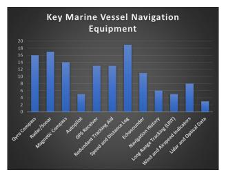
The top five most critical sensing components onboard any vessel are (in order of popularity): speed and distance logs, radar or sonar, gyro compasses, magnetic compasses, and tied for fifth – GPS receivers and redundant tracking aids.
