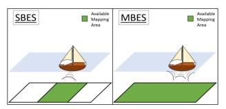
With ping rates of MBESs as high as 50 Hz, you can be confident that regardless of the water depth, when it is paired with an Inertial Labs MRU-PD, acceptable surveying data can be gathered without having to perform numerous passes. The MRU-PD has been tested and works seamlessly with MBES manufacturers like: Teledyne, Klein Marine Systems, Kongsberg, ITER SYSTEMS and NORBIT.
